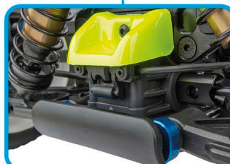
New molded RC8B4.1 front bumper with optimized profile for bumpy transitions
