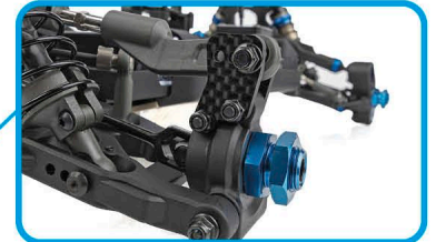
New durable rear hub design with wide footprint base, and tuneable 3mm carbon fiber tall hub towers
