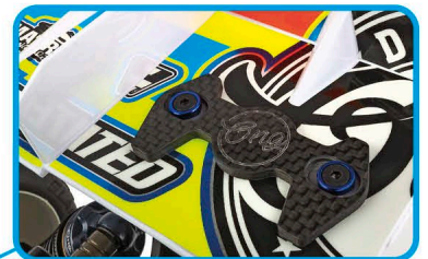
Adjustable wing with official ONG wing mount support, wing button and hardware
